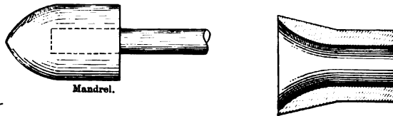
FIG. 237. Making Lap-welded Pipe.
